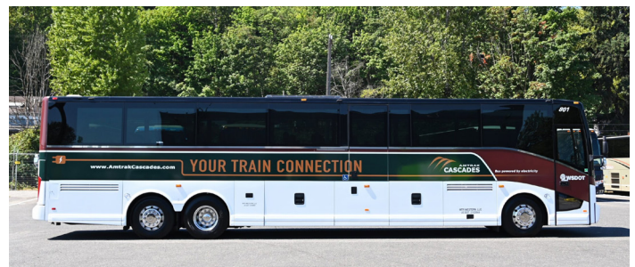
With the Washington State DOT, Amtrak introduced the first-ever electric bus in its Thruway system. This bus makes a nearly 200-mile round trip on a single charge and is estimated to save about 10,000 gallons of diesel fuel per year.
